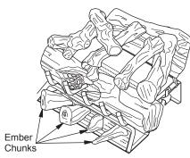
Figure 9 - Placement of Top Logs
